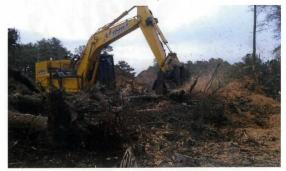
This machine is a one stop shop for many land clearing needs it does the cutting chopping and grinding of trees, stumps and debris leaving just mulch behind. On site disposal of debris means no burning, no trucking, and no dump fees. These machines disperse material that's is ready to walk or drive on.
